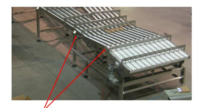
•Infeed line and Stacking device realized with angled belt conveyors and control photocells
