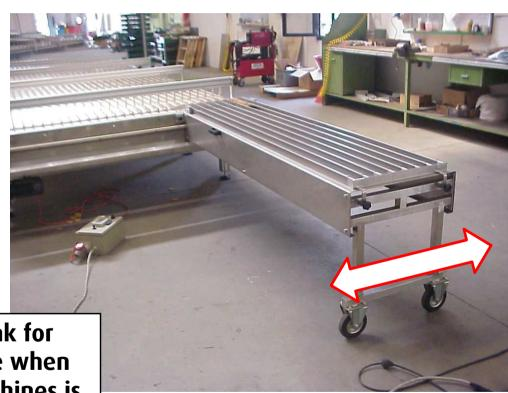
Adjustable position bank for manual packaging to use when one of the flow-wrap machines is bypassed
