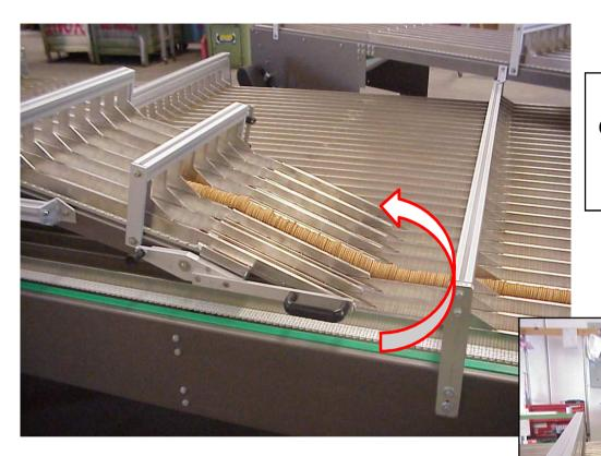
Tilting end for extraction conveyors to allow the bypass of flow-wrap machines in case of stops and failures
