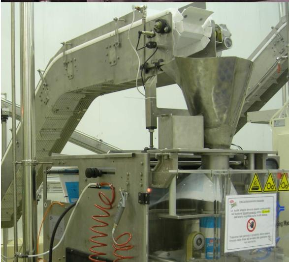
M.H. design, build and install clamp elevators for use in the food industry suitable for any product and environment.
