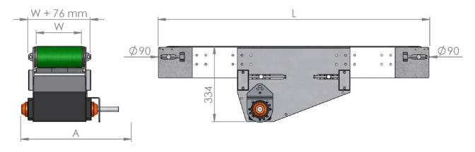
W = Belt width A = Volume depending to the motor gear type L = Conveyor length
