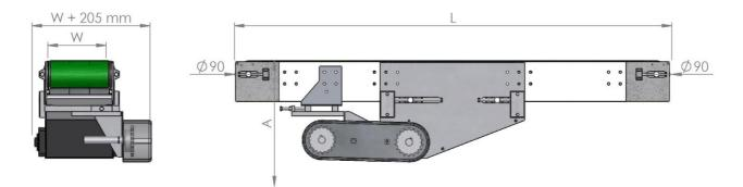
W = Belt width A = Volume depending to the motor gear type L = Conveyor length
