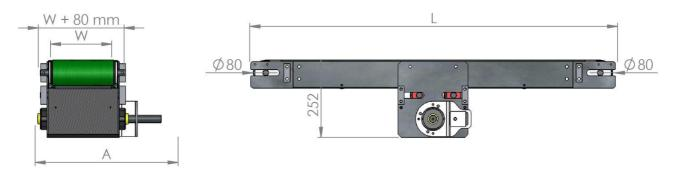
W = Belt width A = Volume depending to the motor gear type L = Conveyor length
