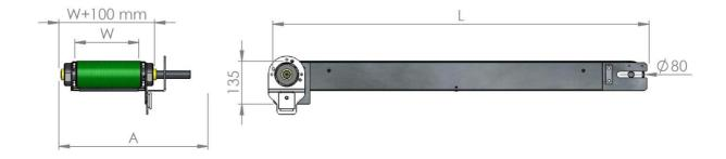
W = Belt width A = Volume depending to the motor gear type L = Conveyor length
