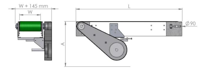
W = Belt width A = Volume depending to the motor gear type L = Conveyor length
