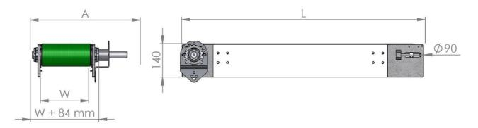
W = Belt width A = Volume depending to the motor gear type L = Conveyor length
