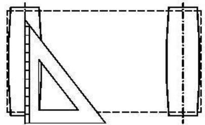
Start-up the unloaded conveyor. Tension the side where the belt is drifting to by acting on the adjustable plates as shown in picture.
