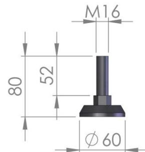
Material : Galvanized steel and rubber
