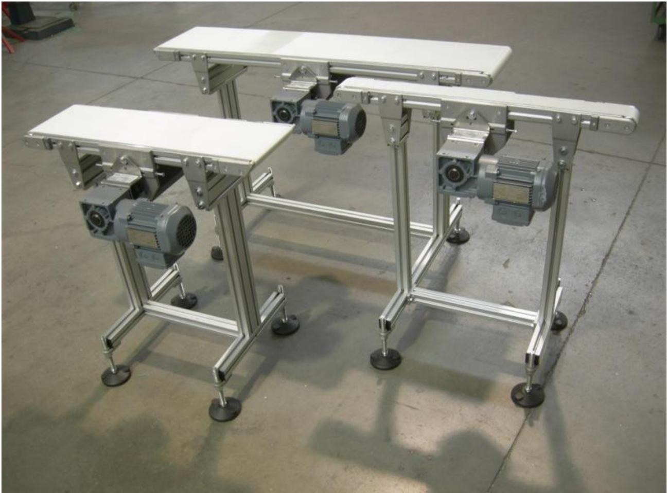
**Suitable for the transportation of light product and with small dimensions, has a maximum work load of 30 Kg\*.
