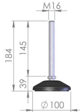
Material : Galvanized steel and Polyamide
