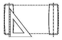
Start-up the unloaded conveyor. Tension the side where the belt is drifting to by acting on the adjustable plates as shown in picture.
