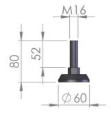
Material : Galvanized steel and rubber
