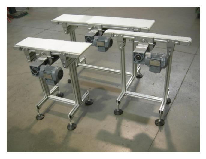
Suitable for the transportation of light product and with small dimensions, has a maximum work load of 30 Kg\*. Its speed can reach 60 m/min\* in function of the installed motor gear and the conveyor dimensions.
