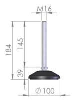
Material : Galvanized steel and Polyamide
