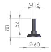
Material : Galvanized steel and rubber
