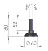
Material : Galvanized steel and rubber
